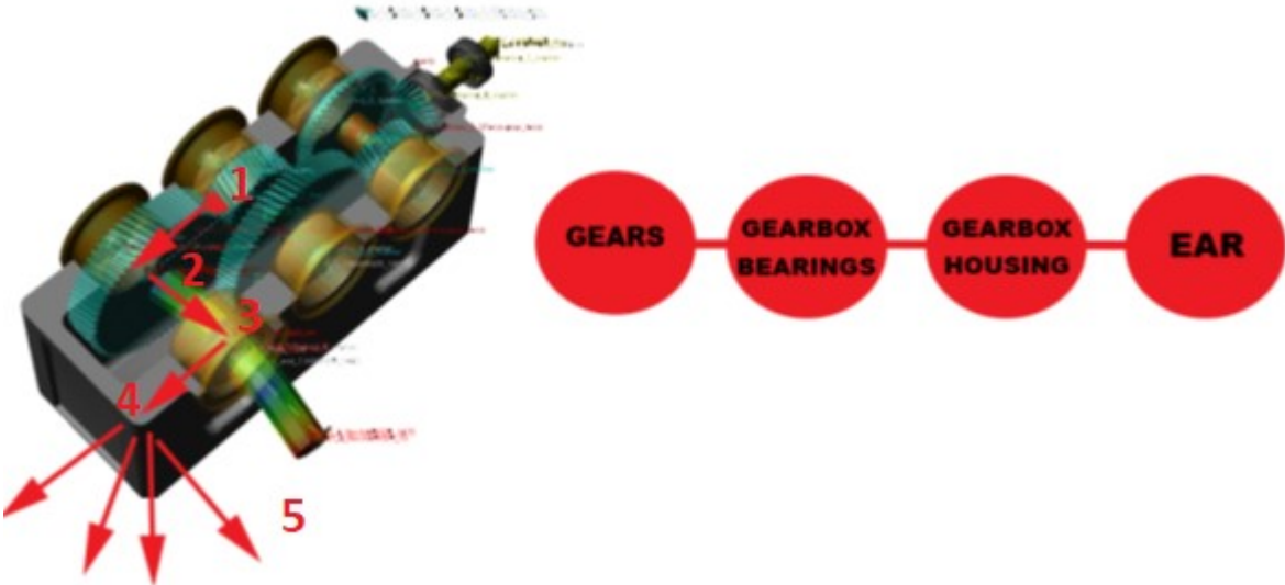
Figure 2. Typical transmission path in gearboxes
